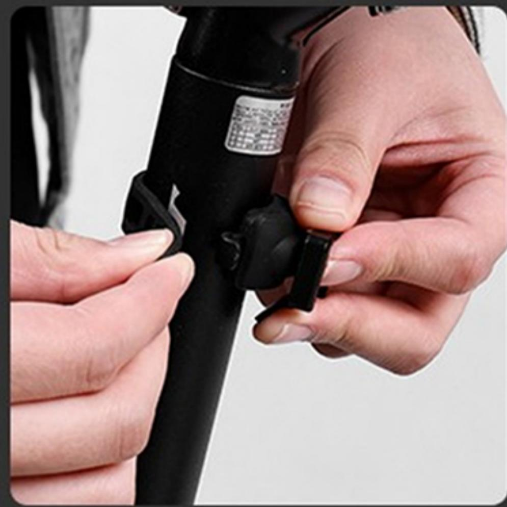
Secure the base to the seat tube
