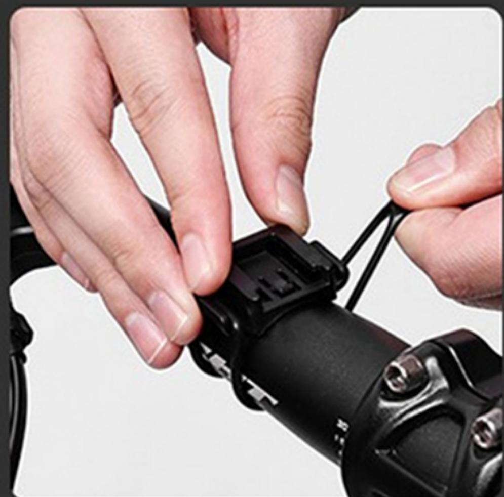
Secure the base to the handlebars with silicone straps
