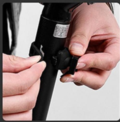
Secure the base to the seat tube
