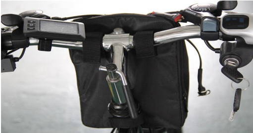
The battery bag is fixed correctly
